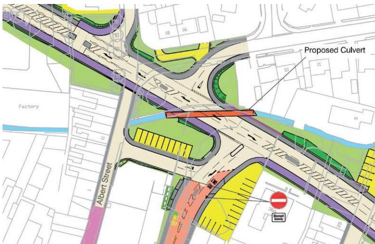
Figure 1 Example of original design with proposed culverting
